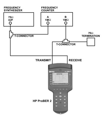
**3** Press **Tx/Rx Setup** and set the display as below.
