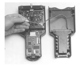
Remove the retaining plate and keep the foam packaging for re-use.
